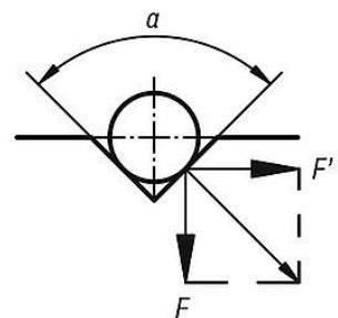
$$\begin{aligned} \alpha = 60^\circ, F' &= 1,732 \times F \\ \alpha = 90^\circ, F' &= F \\ \alpha = 120^\circ, F' &= 0,577 \times F \end{aligned}$$
